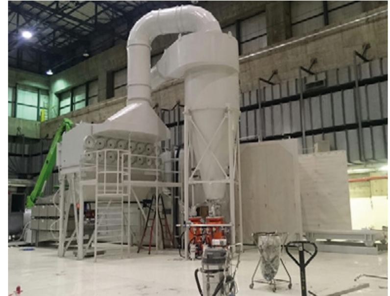
The PULSATRON H cartridge filter is a Pulse-Jet type self-cleaning modular dust remover with pneumatic cartridge cleaning via a puff of counter-current compressed air.
